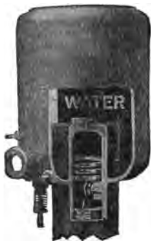
FIG. 177.—The Cylinder and Water Jacket (in section) of a Gas Engine. Designed to prevent premature ignition of the mixture and to assist in lubricating the piston. The water surrounds the cylinder in the section marked "Water."
